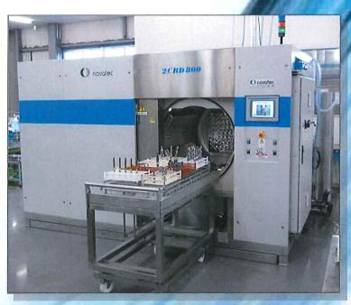
Waterbased System with Basket ROTATION and TILTING
